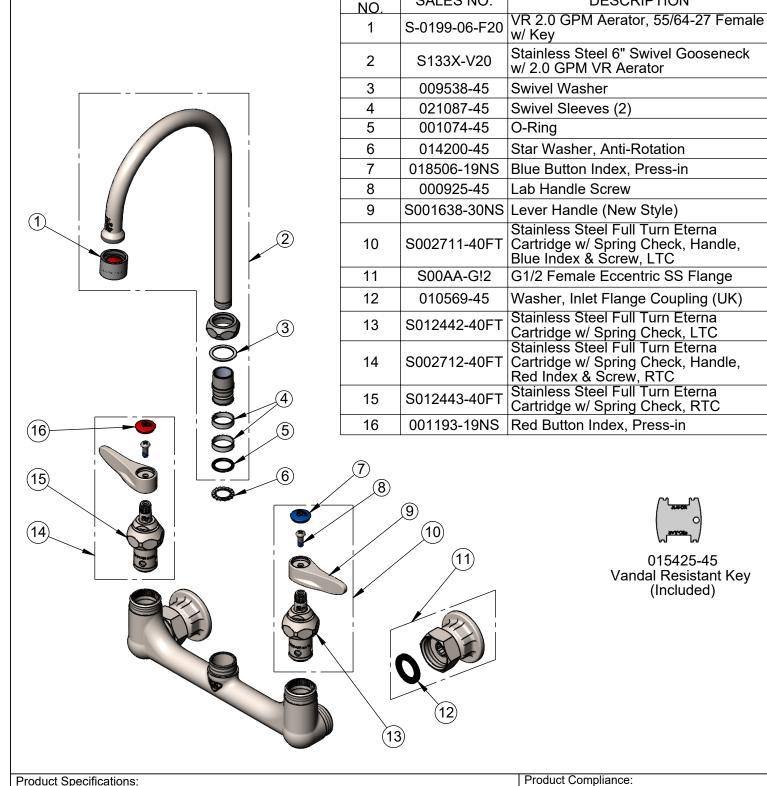
8" Stainless Steel Wall Mount Mixing Faucet, Stainless Steel Full Turn Eterna Cartridges w/ Spring Checks, Stainless Steel Lever Handles, 6" Stainless Steel Swivel/Rigid Gooseneck w/ 2.0 GPM VR Aerator & G1/2 Female Inlets
